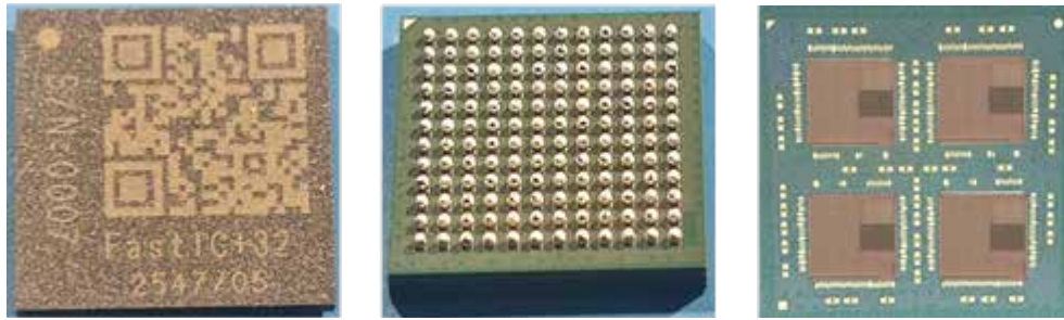
FastIC 32 BGA System in Package and PoETIC 16 channel ASIC block diagram
